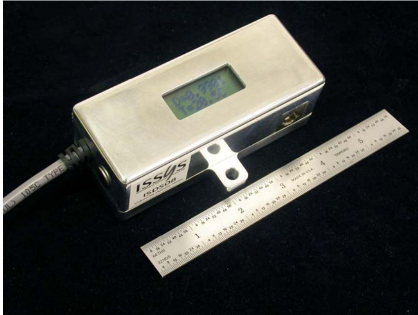
Figure 7. The intrinsically safe ISDS-08 density sensor.
