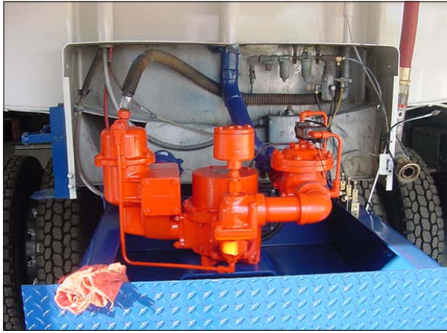
T-11J Meter with T-2A Air Eliminator, Set Stop Valve Electronic Preset Counter and Printer not shown Model T-11J-ZE
